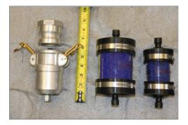
Pindell Engineering LCC is in the world marketplace now with three types of H2Out Systems filters that pull air out of fuel and fluid: a filter for hydraulic systems (left), a large in-line fuel filter and a small in-line filter. These are made in Jefferson County with components brought in from around the world. Photos by Patrick J. Sullivan
