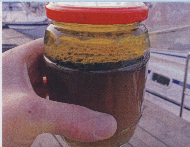
Here's a sample of the sort of bacteria that can grow in your fuel once it is contaminated with water
